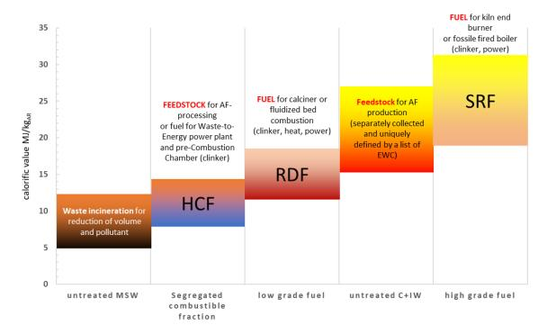
With regard to the envisaged valorization process several qualities shall the derived from waste. For the process of clinker burning and production of electricity there are several terms and specifications:
