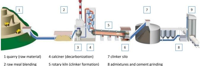
2 raw meal blending 5 rotary kiln (clinker formation) 8 admixtures and cement grinding
