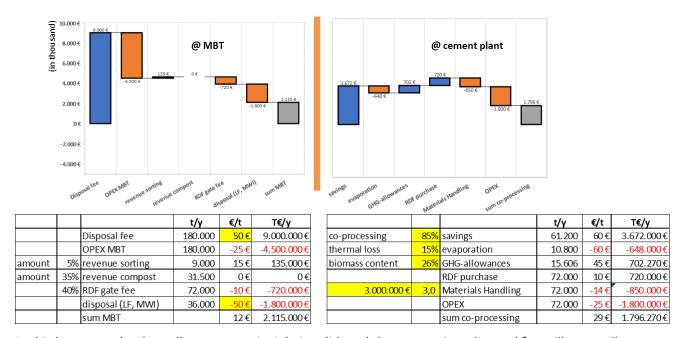
In this last example, the polluter-pays-principle is valid, and the appropriate disposal fee will cover all the investment into a suitable technology to produce RDF with a suitable quality. The cement plant will extend its reception and storage facility to guaranty a continuous supply and will get a gate fee to compensate its higher investments such as SCR- or SNCR-technology to reduce  $NO_x$ -emissions.
