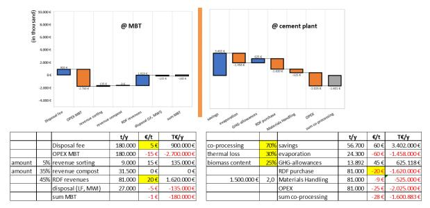
By a quick review of the calculations, this project to producing alternative fuels in a simple MBT will fail, even despite financial support from the cement plant.
