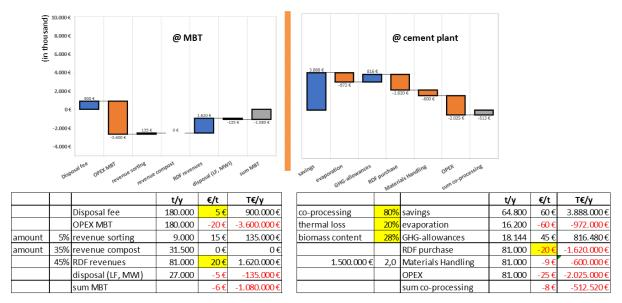
On one hand, upgrading the MBT will generate a better RDF quality with a higher biomass content and a lesser introduction of moisture, and consequently a higher thermal substitution rate at the cement plant. Its losses will be halved, but will still remain negative.
